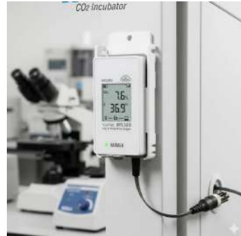
VaiNet wireless CO2 data logger RFL100
