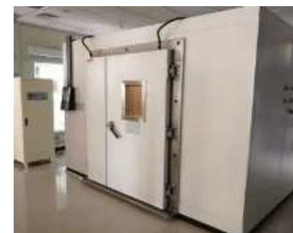
Walk-in Low Temperature Room
