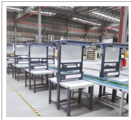
Belt Conveyor with Work Table
