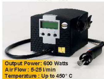
Programmable Hot Air Rework Tool HCT - 1000
