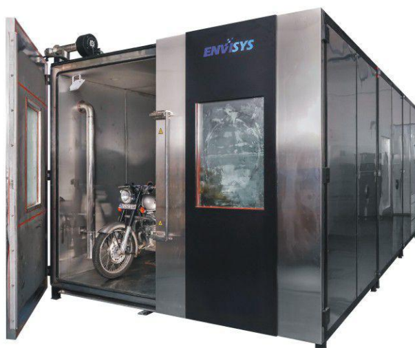
Drive-in Test Chamber
