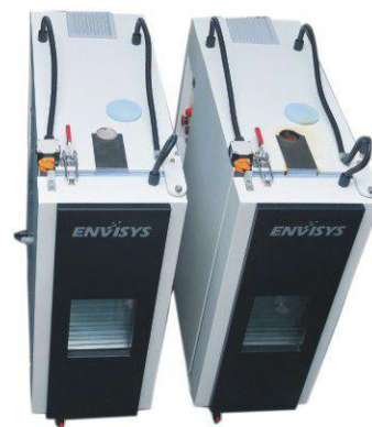
Top and Bottom of the chamber for interfacing with UTM interfacing slots and cover
