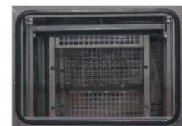
SS Specimen Carrying Test Basket
