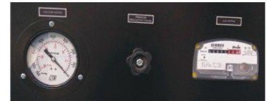
Vacuum Flow-Meter and Regulation
