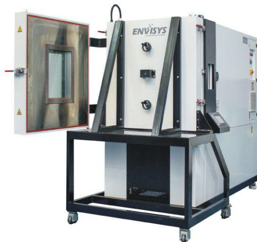
Environmental Test Chamber for skid mounted door fixing provision to test P4 speed sensors
