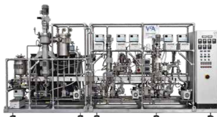
Multistage Unit with One Wiped Film Evaporator, Two Short Path Evaporator and degasser
