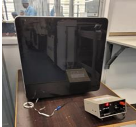
Solder Paste - Storing & Temp. monitoring
