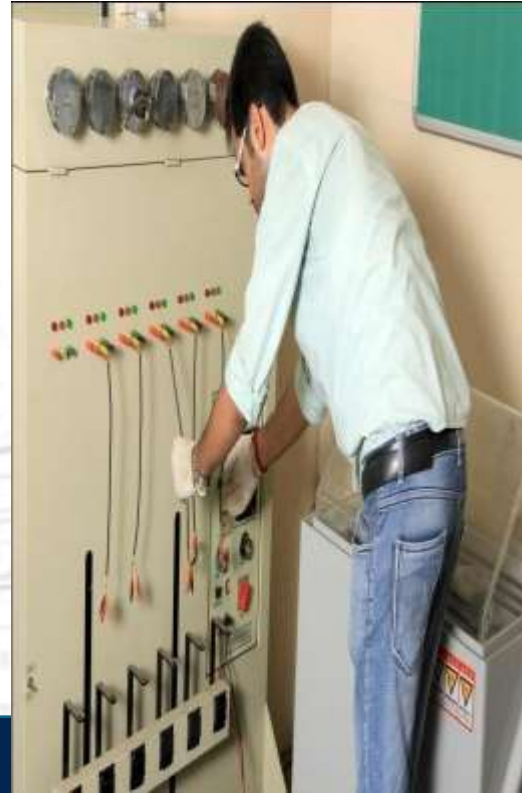
Power Cord Abrupt Pull tester
