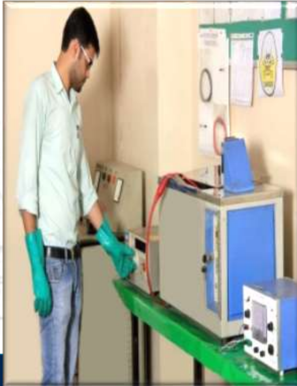
High Voltage & leakage Current Testing Equipment
