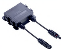
1070-9 4-rail, with diodes, 12A potted/ 10A non-potted, IP67, TUV
