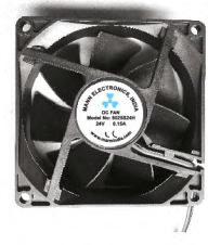
MN-9071-2, 9025S24H DC FAN 90×90×25, 0.15A, 24V, 2 PIN WITH CONNECTOR (205), RPM 2800, 33.2 db, CFM53.1
