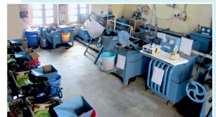
FINISHING SHOP WITH ALL PLATING FACILITY LIKE ULTRASONIC AND ELECTROLYTIC CLEANING, LABORATORY, THICKNESS TESTER, SALT SPRAY CHAMBER, CORROSION TESTING ETC
