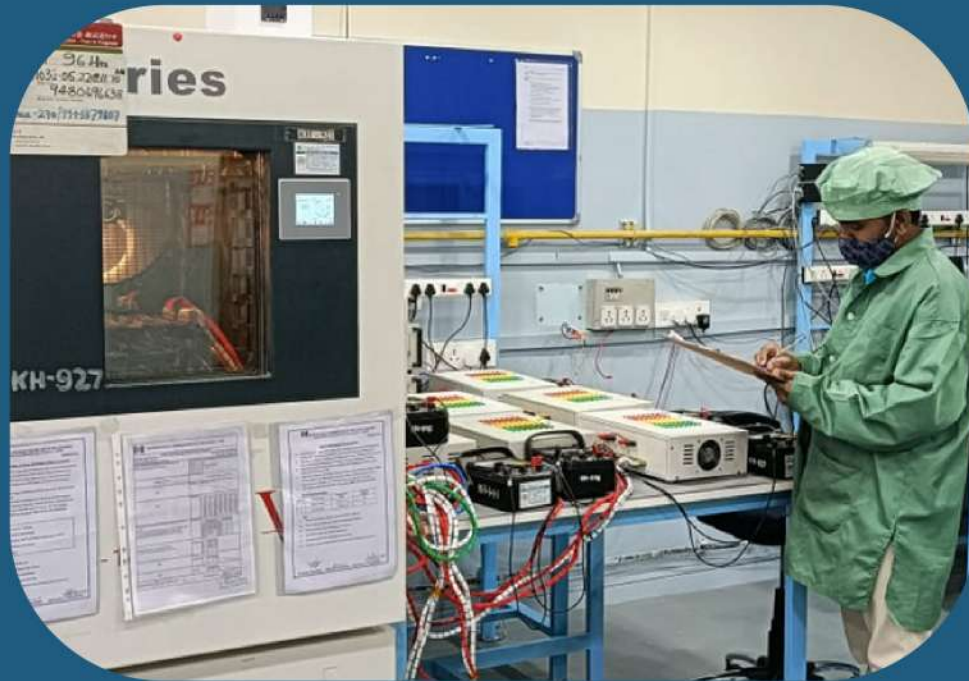
Burn-In & ATC Chambers: -40^{\circ}\text{C} to +180^{\circ}\text{C}
