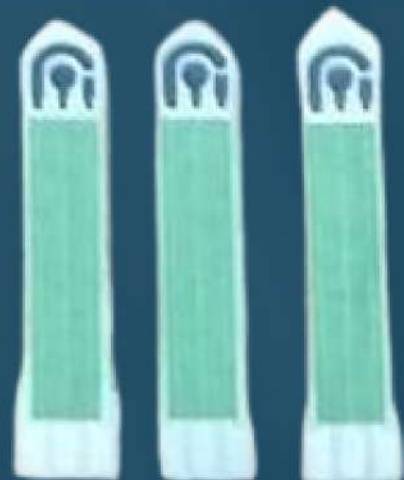
CERAMIC BASED SENSING ELECTRODES
