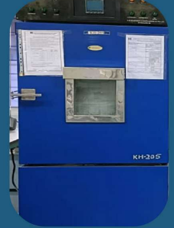
Cold Chamber @ -65^{\circ}\text{C}
